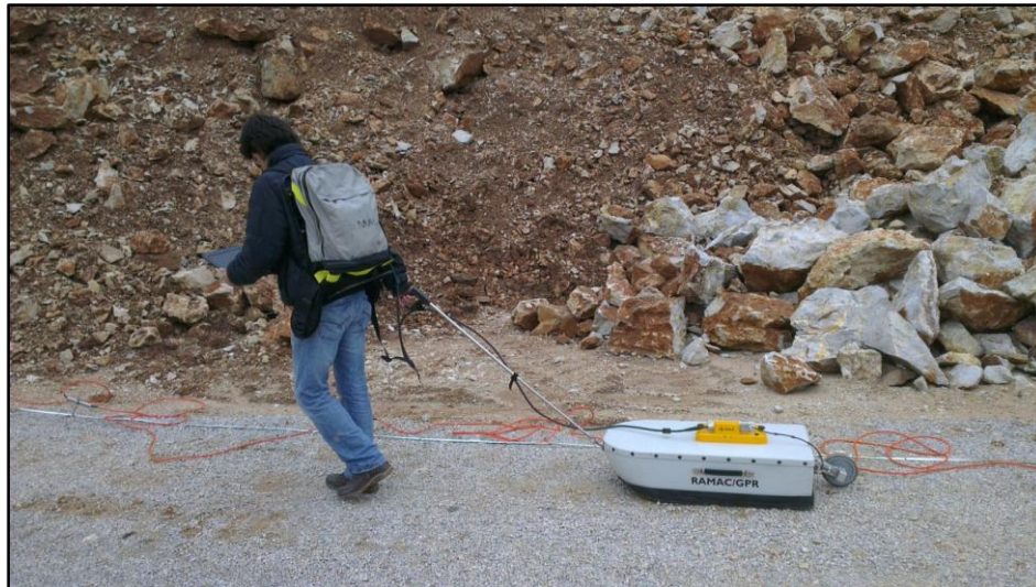
Figure 6: Ground Penetrating Radar (GPR) measuring device and its use during field surveying
