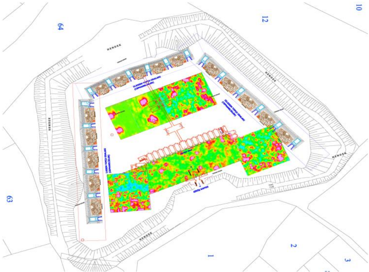
Figure 9: Application of analytical signal belonging to bastion
