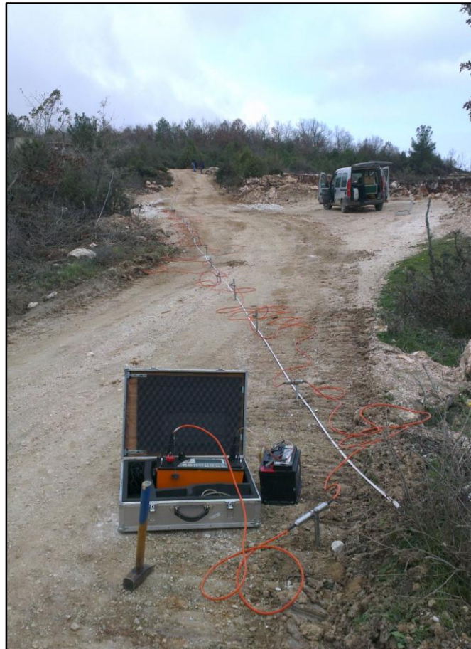
Figure 3: Electrical Resistivity field application
